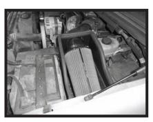
Step 11 Install the filter and fasten it securely.
